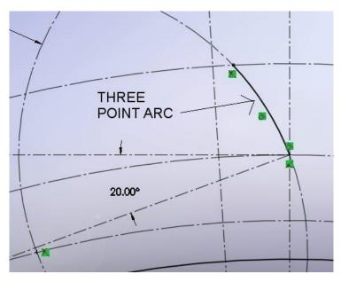
9. Now sketch a Tangent Arc named the Bottom Arc. This arc will represent the bottom surface of one of the gear teeth. Start this arc at the bottom end point of the 3 Point Arc - sketched in the previous step – with the second endpoint coincident to the Root Diameter circle. This arc needs to be perpendicular to the Root Diameter circle (which will be covered in the next step). Refer to the image nearby.
